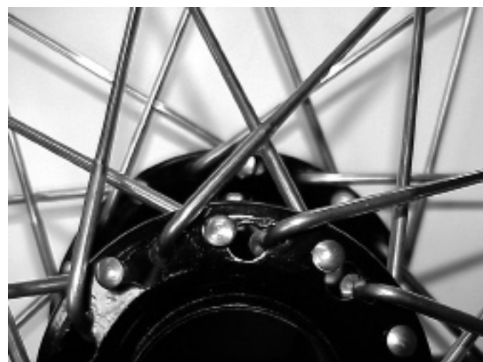
Photo #7: The last set of 10 37-1108 spokes lace in the “keyhole” flange. First spoke goes cw from the inside in the open side of the keyhole and 7 holes cw from the valve stem. After lacing the first spoke in the referenced keyhole move to the next open keyhole and four holes over in the rim.
