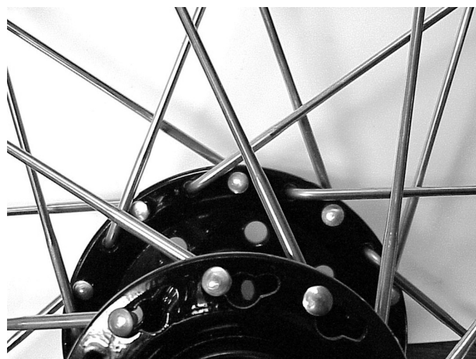
Photo #6: The third set of 10 37-1108 spokes lace in the “keyhole” flange. The first spoke goes ccw from the outside into the marked “keyhole” and 8 holes ccw from the valve stem. After lacing the first spoke in the referenced keyhole move to the next keyhole and four holes over in the rim.
