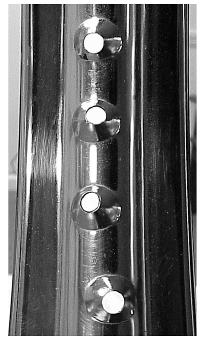
37-7030 1976-up Rear rim with "3 by 1" dimpling— 3 dimples on left sprocket) side of rim and one on the right (disc) side. This rim is handed.
