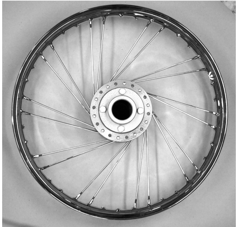
Front Disc Wheel Viewed from Left Side (non-side) all inside spokes radiate clockwise.
