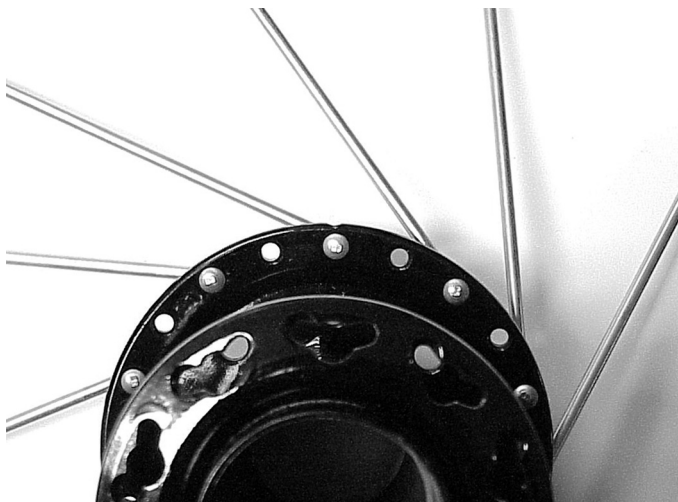
Photo #4: First set of 10 37-3402 spokes laced in the “brake drum” flange. First spoke goes ccw from inside into marked hole in hub and 7 holes ccw from valve stem. After lacing first spoke in referenced hole move two holes in the hub and four in the rim and install the next spoke.
