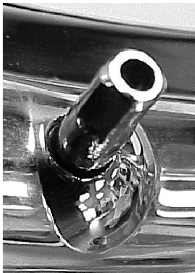
A Triumph rim pierced to accept a .300 inch nipple with a smaller .281 inch nipple. I show this because in the US .281 inch Japanese style nipples often find their way into Triumph spoke kits. It is possible this nipple could pull through during tightening, or fail in use, it is important to be sure you use the correct nipple for your rim.
