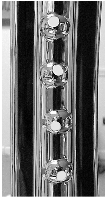
37-1230 19 to 1970 Front rim with alternative "2 by 2" dimpling— 2 dimples on the left then 2 on the right. This rim is not handed.
