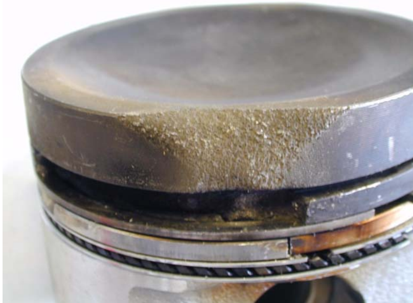
Ignition occurs from hot deposit.
